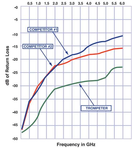
NOTE: Test setup includes one foot Belden 1505A coaxial cable with BNC plug each end plus adapter and termination.
