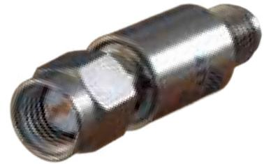
Midwest Microwave's SMA miniature series of fixed coaxial attenuators provide temperature stable, ruggedly built, precision performance in a small light weight package size. Attenuation values 0 - 30 dB are available with any of the units described and with male to female SMA connectors.
