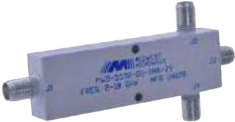
Midwest Microwave’s series of high performance isolated Three Way Power Dividers are true three way dividers. They are small, lightweight, ruggedly constructed stripline units that possess inherently low insertion loss and VSWR with high isolation and excellent phase and amplitude tracking. Units are available in ultra-wideband frequency bandwidths covering the entire range of 2.0 - 18.0 GHz.
