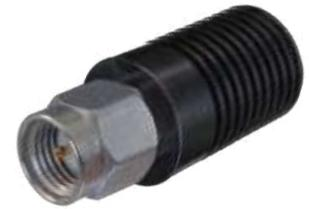
Midwest Microwave's SMA series of medium power coaxial Terminations provide temperature stable, ruggedly built, precision performance in light weight reasonably sized packages using stainless steel connectors and black anodized finned aluminum housings. Input Power levels of 10 and 20 Watts are offered with low VSWR performance. Contact factory for custom versions and different configurations.
