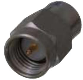
Midwest Microwave's series of Short and Open Circuits are conveniently offered in all of the popular male and female connector interfaces. They are particularly useful for performing phase measurement tests. The units are finished in passivated stainless steel. Contact factory for custom versions and different configurations.
