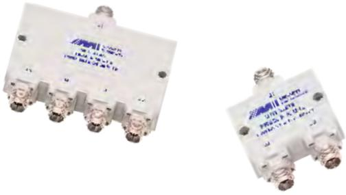
Midwest Microwave 40 GHz power dividers are small, lightweight, and ruggedly built. They cover a wide bandwidth of 6-40 GHz with low insertion loss and low VSWR. Power dividers use Wilkinson design for the lowest insertion loss and the highest isolation. They use 2.92mm female stainless-steel interface and are built in aluminum housing coated with gray paint.
