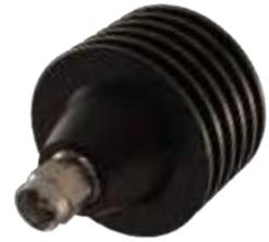
Midwest Microwave's SMA series of medium power coaxial Terminations provide temperature stable, ruggedly built, precision performance in light weight reasonably sized packages using stainless steel connectors and black anodized finned aluminum housings. Input Power levels of 3, 5, and 10 Watts are offered with low VSWR performance. Contact factory for custom versions and different configurations.
