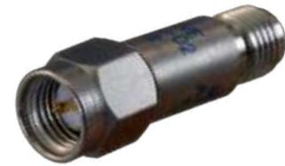
Midwest Microwave's SMA subminiature series of fixed coaxial attenuators provide temperature stable, ruggedly built, precision performance in a compact lightweight package size. Attenuation values up through 30 dB are available with any of the units described and with specified combination of female or male SMA connectors.
