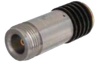
Midwest Microwave's Type N series of medium power coaxial Terminations provide temperature stable, ruggedly built, precision performance in light weight reasonably sized packages using stainless steel connectors and housings of black anodized finned aluminum for maximum heat dissipation. Input Power levels of 10 Watts is offered with low VSWR performance. Contact factory for custom versions and different configurations.
