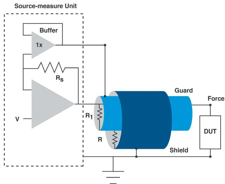
The capacitive effects of cable insulation should also be considered. If the test schedule requires the applied voltage to be swept, this parasitic capacitance will draw a charging current in proportion to its magnitude and the rate of change of applied voltage ( $I_c = C \, dV/dt$ ).
