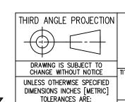
TOLERANCES ARE: ANGLES ± 2° 1 PLC. DEC. ±.010" [±0.25] 2 PLC. DEC. ±.008" [±0.20] 3 PLC. DEC. ±.006" [±0.15] DO NOT SCALE DRAWING 1 OF 2
